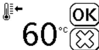
After defining the desired working mode (14), it may make sense to adjust the pre-heat temperature of the programme temperature. This avoids long heat-up or cool-down phases.
