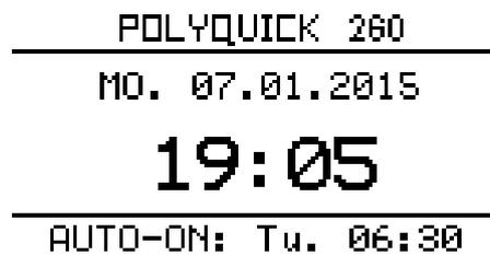
When you press the Sleep button, the device goes into the Sleep mode (all functions except the Timer function are switched off). The device gets actuated when you press the touch display or with the timer and heats up or cools down to the preset pre-heating temperature.
