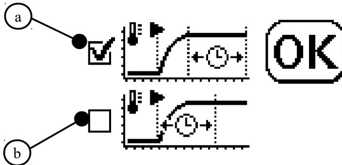
(a) (Default) The device heats to the temperature programmed under **6**. After reaching this value, the result measured is validated by a control cycle. If the value is confirmed, the wax polymerisation process will start.
