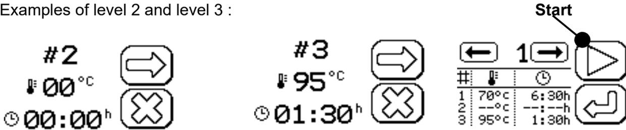
Touch the arrow (Start) to start the process of polymerisation.
