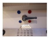
Ball valve: For the blasting process the selection lever must be in a horizontal position!
