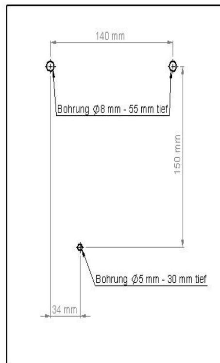
Secure the enclosed screw anchors as shown in *Figure 1*. Screw the 6x50 screws into the two upper holes; keep a distance of 6-7 mm to the wall! (*Figure 2*)
